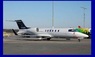
Type:Bombardier Learjet 40Wingspan:47.8'Length:55.6'Max Wt.20,350 lbs.
