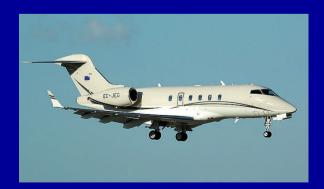
Type:Bombardier Challenger<br/>300 BD-100-1A10Wingspan:63.8'Length:68.6'Max Wt.38,850 lbs.
