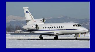
Type:Dassault Falcon 900EXWingspan:63.4'Length:66.3'Max Wt.46,700 lbs.
